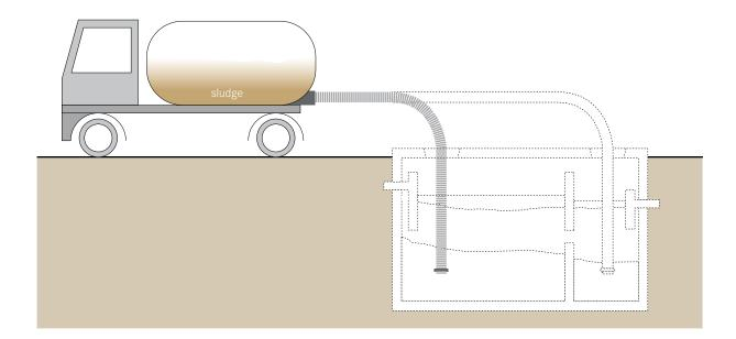
Motorized emptying and transport refers to a vehicle equipped with a motorized pump and a storage tank for emptying and transporting faecal sludge and urine. Humans are required to operate the pump and manoeuvre the hose, but sludge is not manually lifted or transported.
